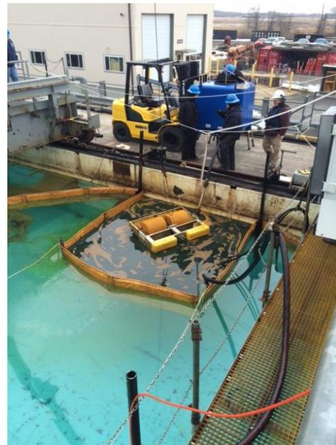
**Image 4:** Recovered oil- (10x10 ft) for recovery test (2/11/2015).
