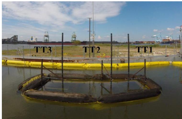
Figure 37. Placement of thermocouple trees during large-scale ISB tests.
