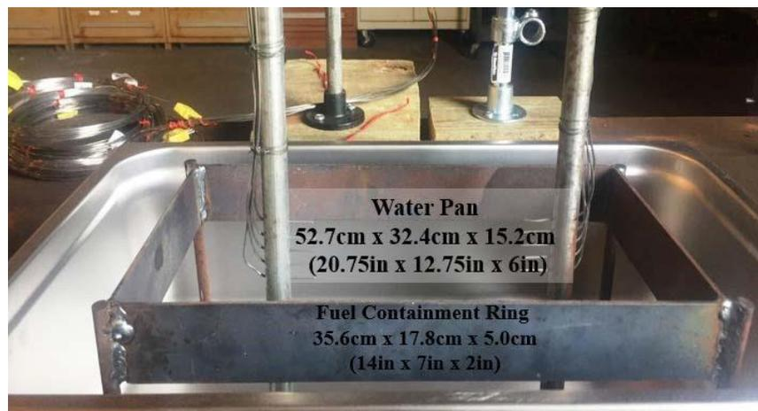
Figure 4. Small-scale test apparatus.
