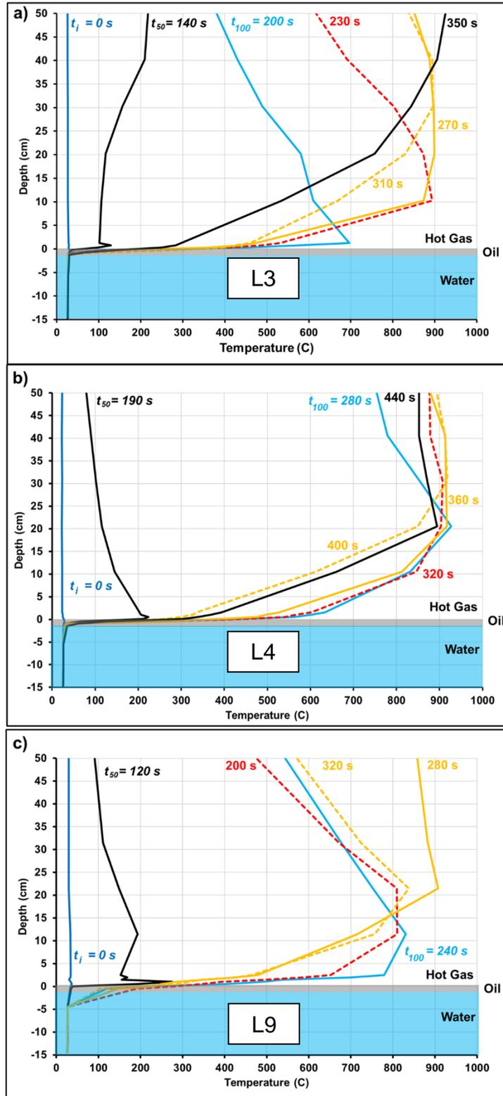
Figure D-5. Temperature profiles of example mesoscale experiments.
