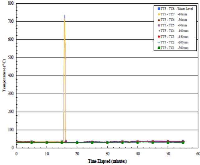
TT3 - Temperature Below Water Level - Test\_01
