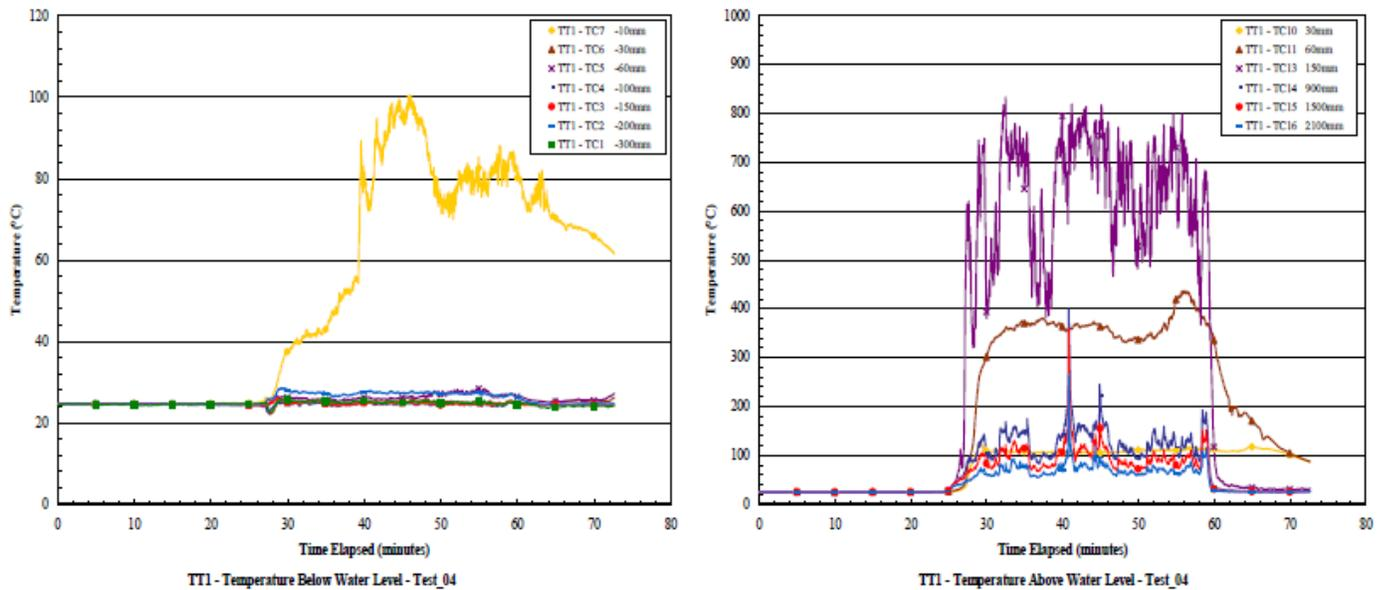
Figure F-12. Large-scale test L4 (RMG 380 with vegetation), thermocouple tree 1.
