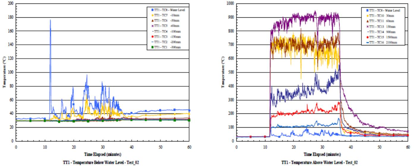
Figure F-5. Large-scale test L2 (crude oil with vegetation), thermocouple tree 1.
