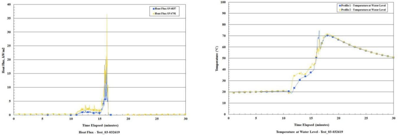
Figure C-4. Test 3 total heat flux measurement and temperature at the water level.
