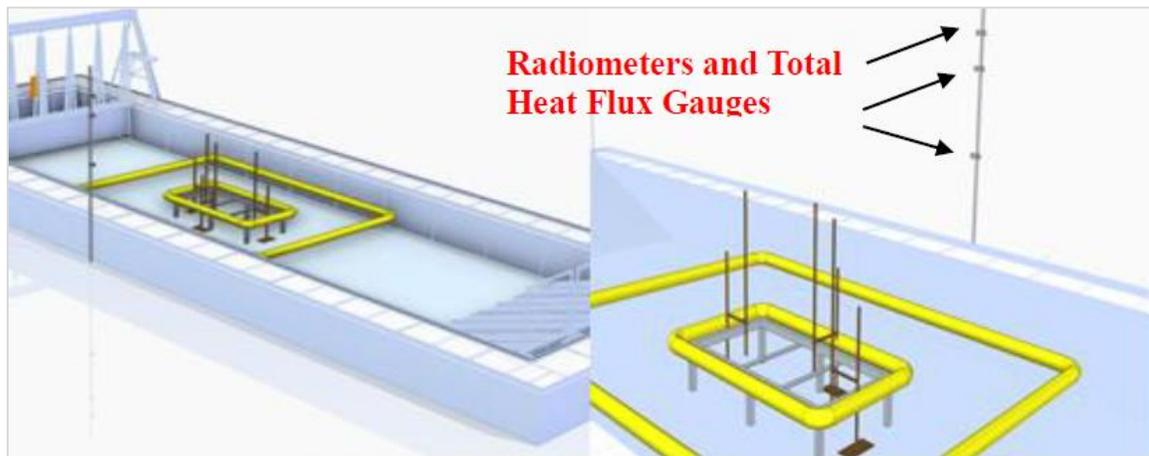
Figure 38. Large-scale ISB heat flux gauge setup.
