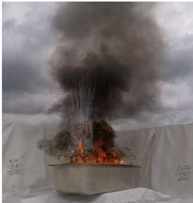
Figure 18. Steam eruptions and fuel oil splatter events during small-scale tests.
