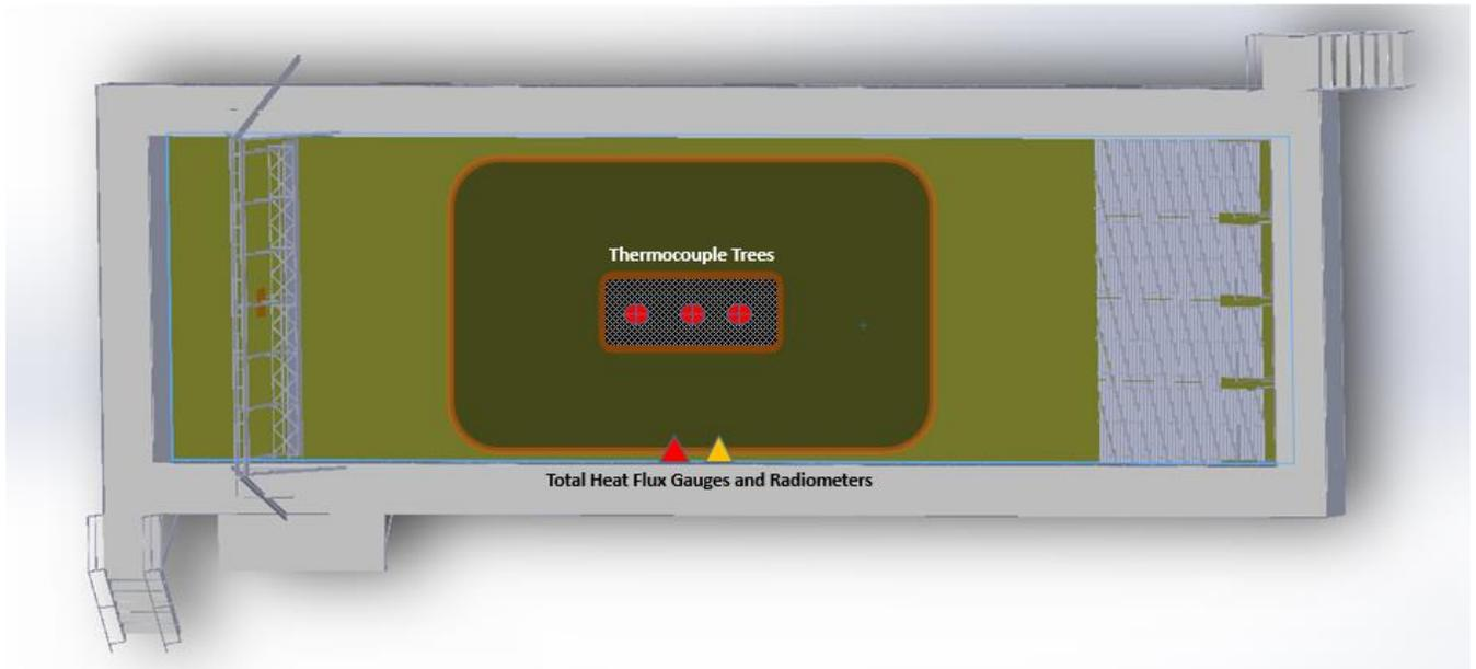
Figure 36. Overview of temperature instrumentation placement for ISB tests. Red circles depict thermocouple trees inside the burn area (primary containment). Heat flux and radiometers are outside the secondary containment.
