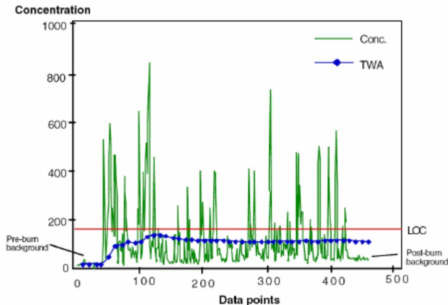
Figure E-1. Sample graph of ISB smoke plume field monitoring data collected via SMART protocol.
