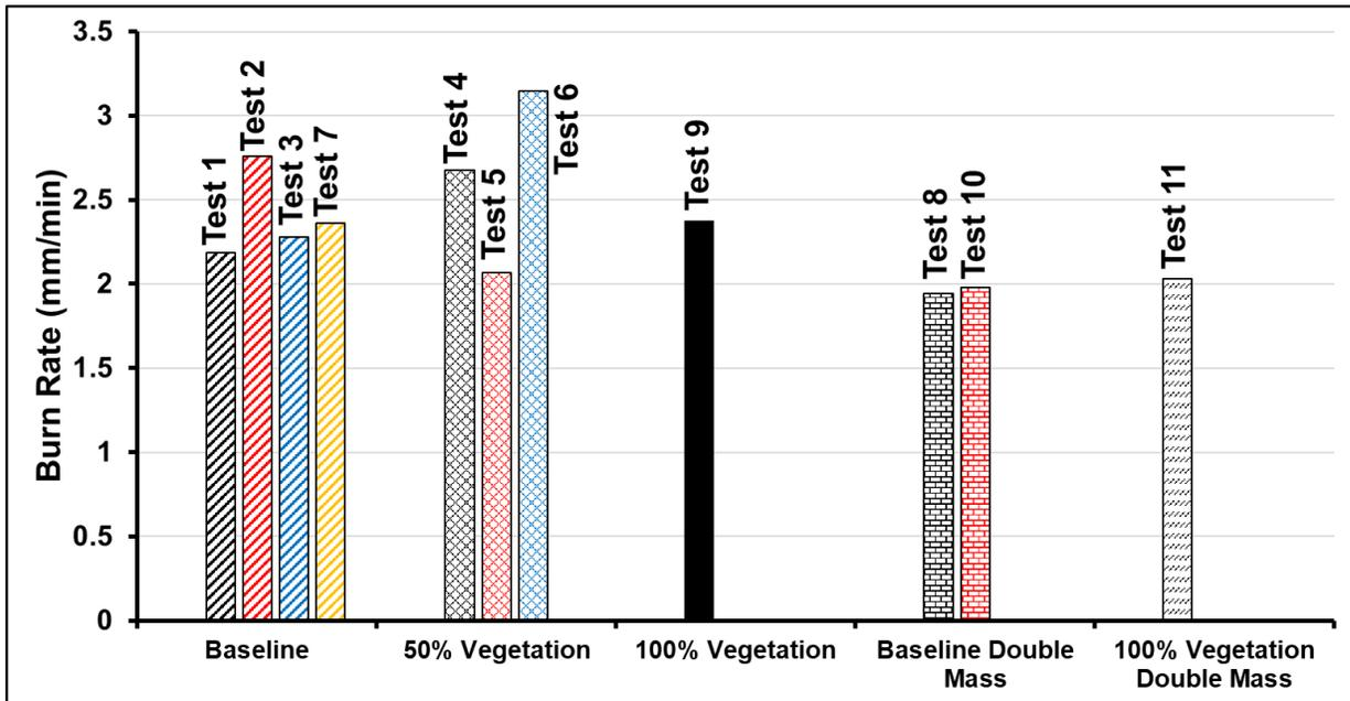
Figure D-4. Experimental burn rates calculated by the area integration method.
