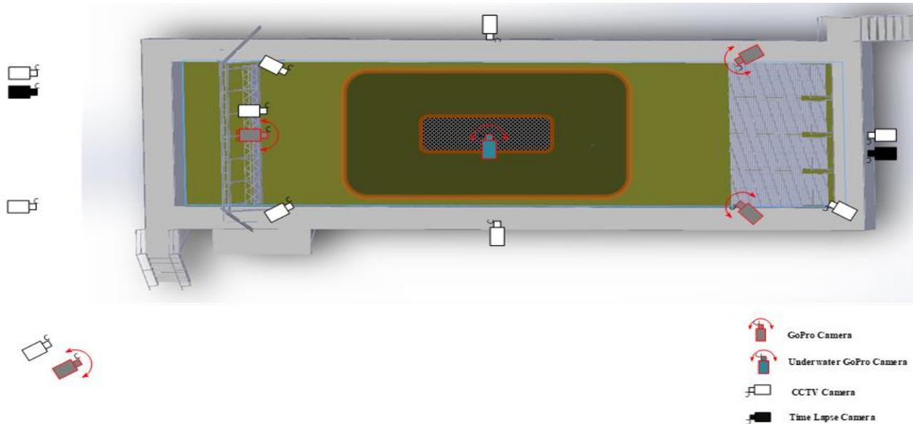
Figure 41. Stationary video placements for large-scale ISB tests.
