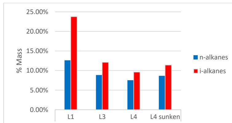
Figure 49. Alkane mass percentages in residue from large-scale ISB of crude (L1 only) and RMG 380.
