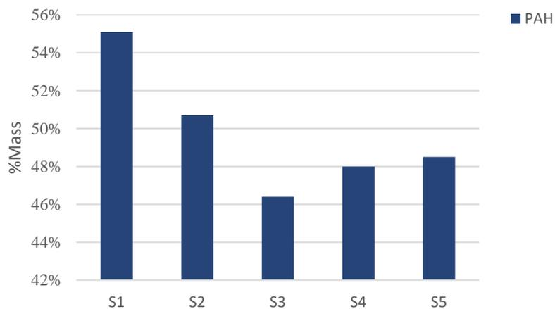
Figure 16. PAH concentrations in post-burn residue
