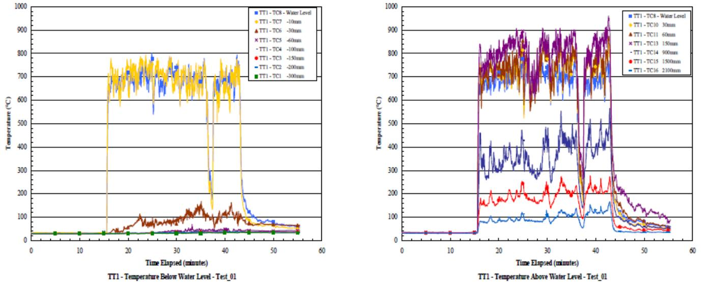
Figure F-1. Large-scale test L1 (crude oil baseline), thermocouple tree 1.
