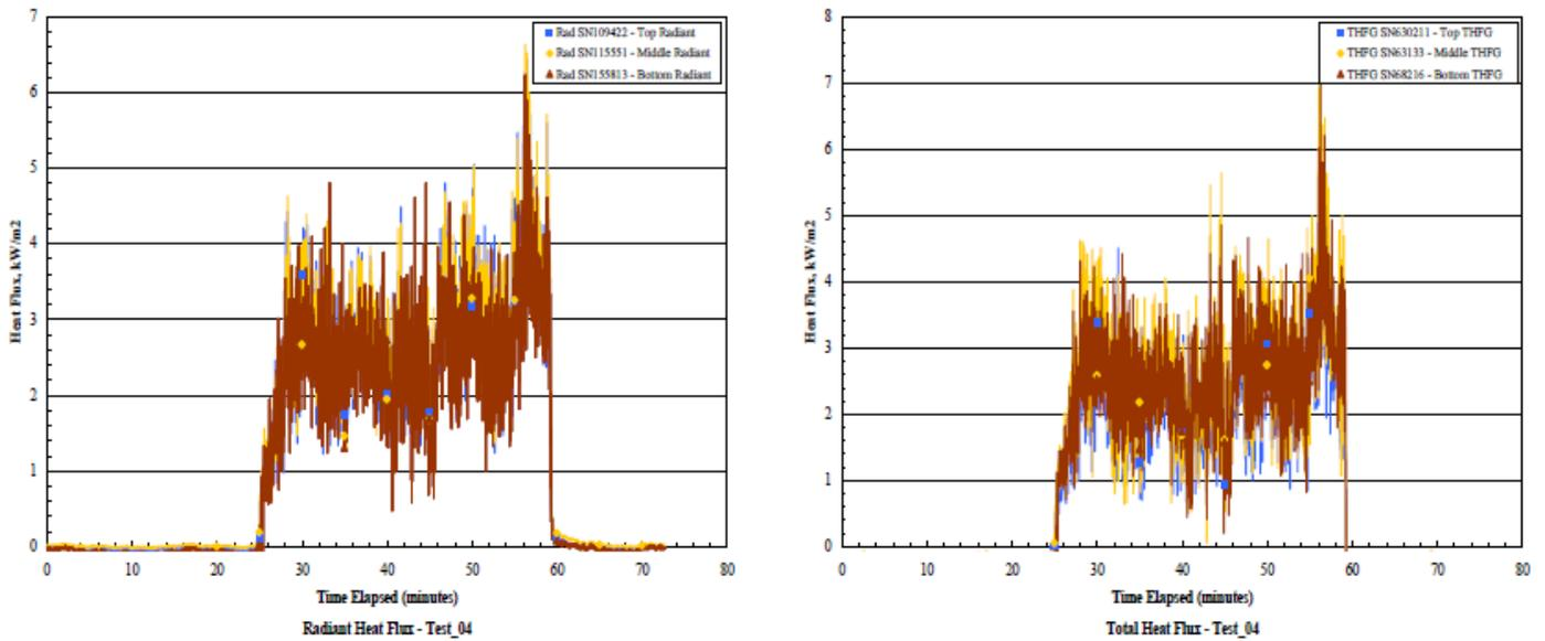
Figure F-14. Large-scale test L4 (RMG 380 with vegetation), radiant and total heat flux measurements.
