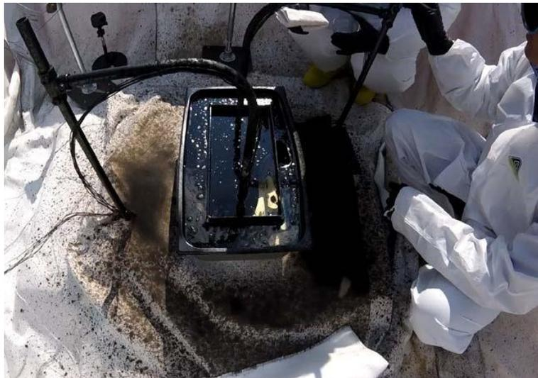
Figure 13. Splattered oily residue around the perimeter of the small-scale burn pan.
