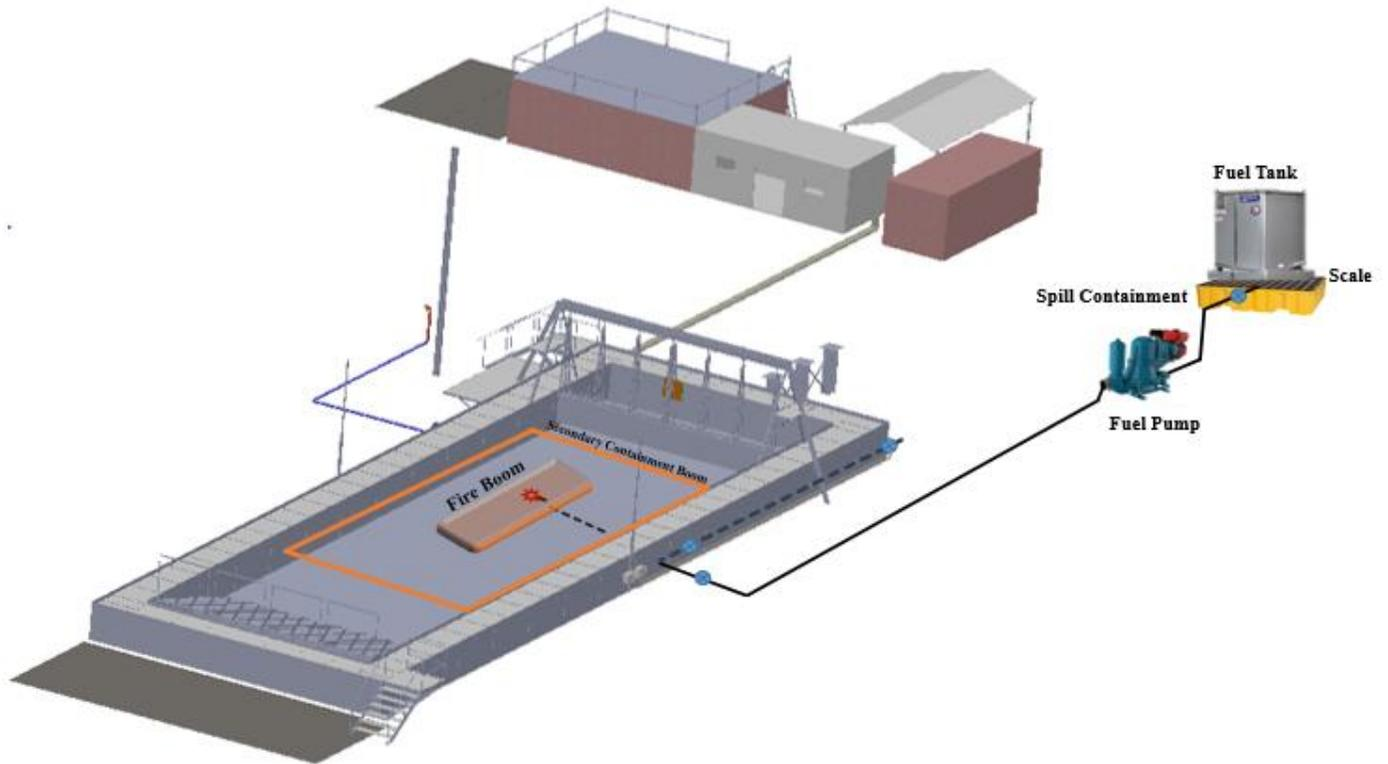
Figure 34. Flowing fuel system large-scale ISB.
