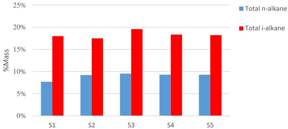
Figure 15. Total n- and i-alkane (C<sub>5</sub>-C<sub>10</sub>) mass percentages in residue from small-scale ISB of RMG 380.
