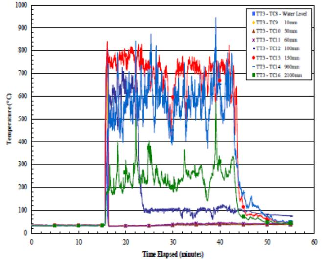
TT3 - Temperature Above Water Level - Test\_01
