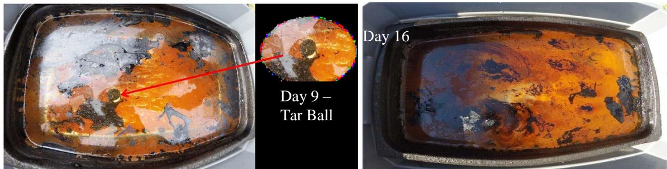
Figure 20. Oil residue and tar balls after nine days and sixteen days of weathering.
