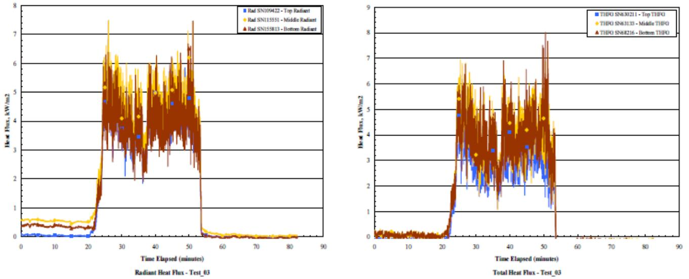
Figure F-11. Large-scale test L3 (RMG 380 baseline), radiant and total heat flux measurements.
