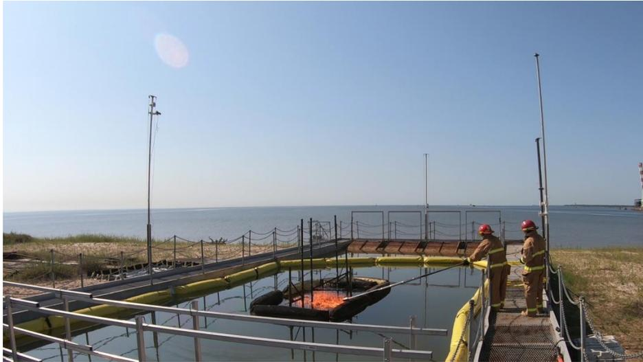
Figure 42. Ignition of large-scale ISB tests using extended torch at JMTF.
