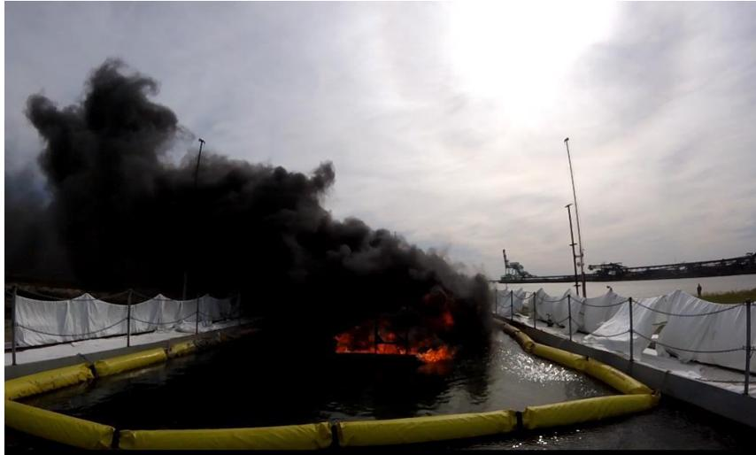
Figure 48. Large-scale flame and low smoke layer (L4).
