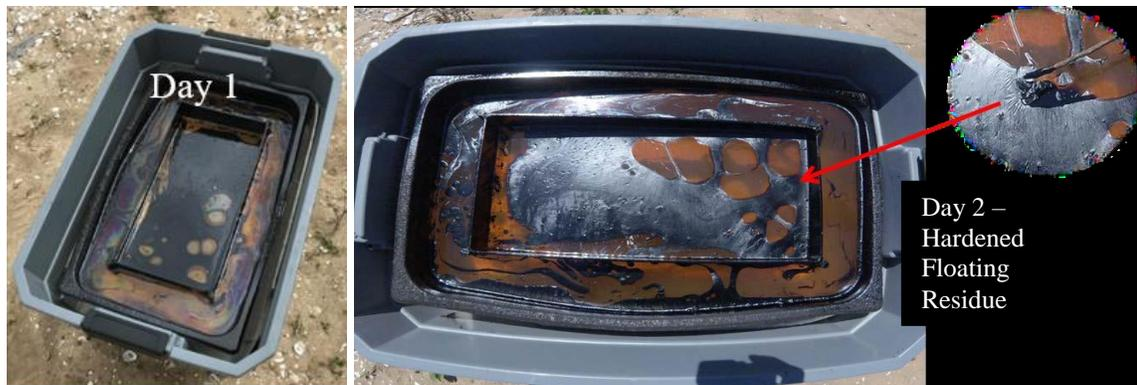
Figure 19. Oil residue after two days of weathering.
