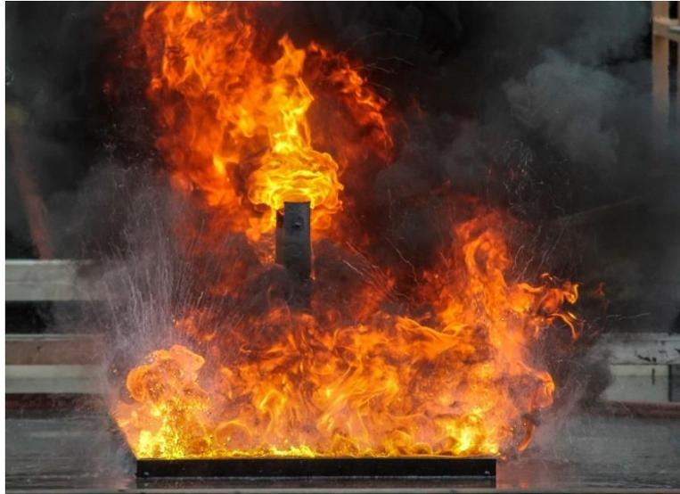
Figure 31. Boil over visible during mesoscale ISB.
