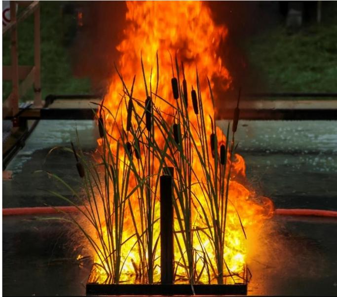
Figure 27. Fully engulfed mesoscale ISB with vegetation.
