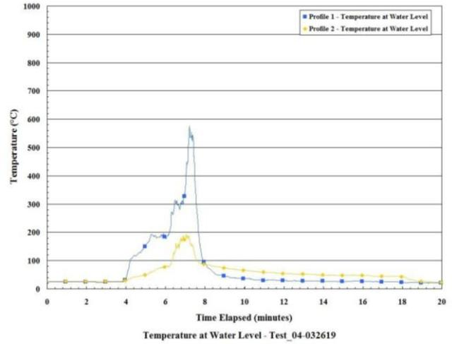
Figure C-6. Test 4 total heat flux measurement and temperature at the water level.
