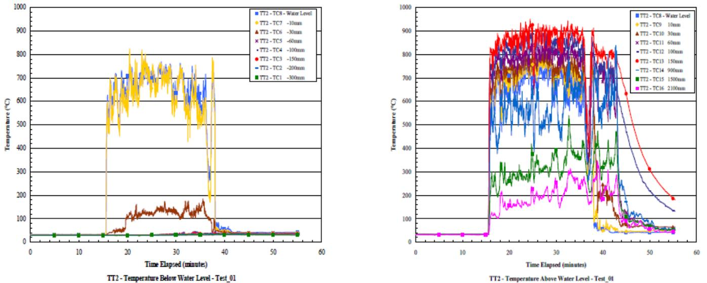
Figure F-2. Large-scale test L1 (crude oil baseline), thermocouple tree 2.
