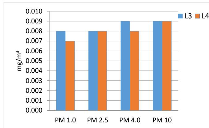
Figure 52. PM size distributions measured by ground-based instrument closest to burn pan.
