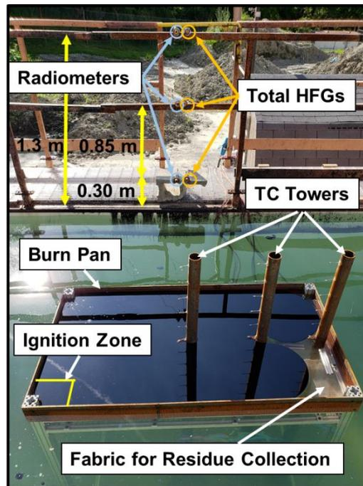
Figure 24. Instrumentation used in mesoscale experiments.
