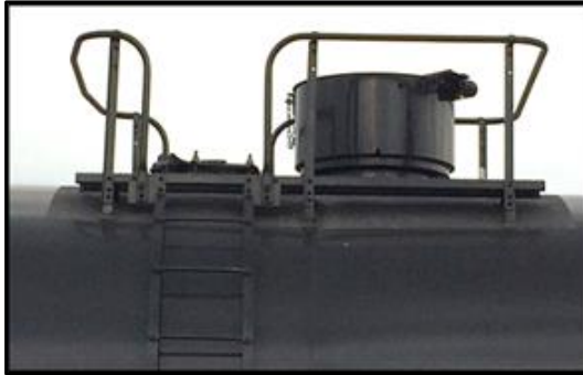
Class DOT/TC-117 Manway and Top Fittings Protective Housing
