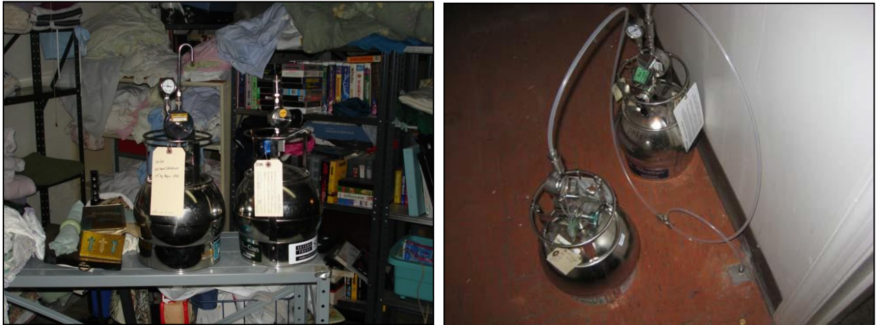
Figure 6-10. Collocated Indoor Air Samples (Left) and Sub-slab Soil Gas Samples (Right)
