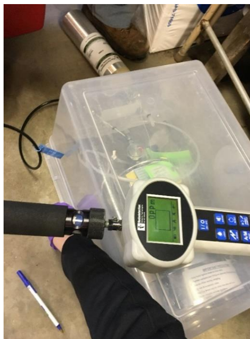
Figure 6-6. Helium Leak Test Using Shroud
