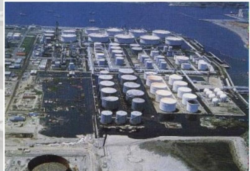
Figure 9. Spilled oil inundated a refinery area in Sendai at the 1978 Miyagi Earthquake (Courtesy of Kahoku Simpo Publishing Co.)
