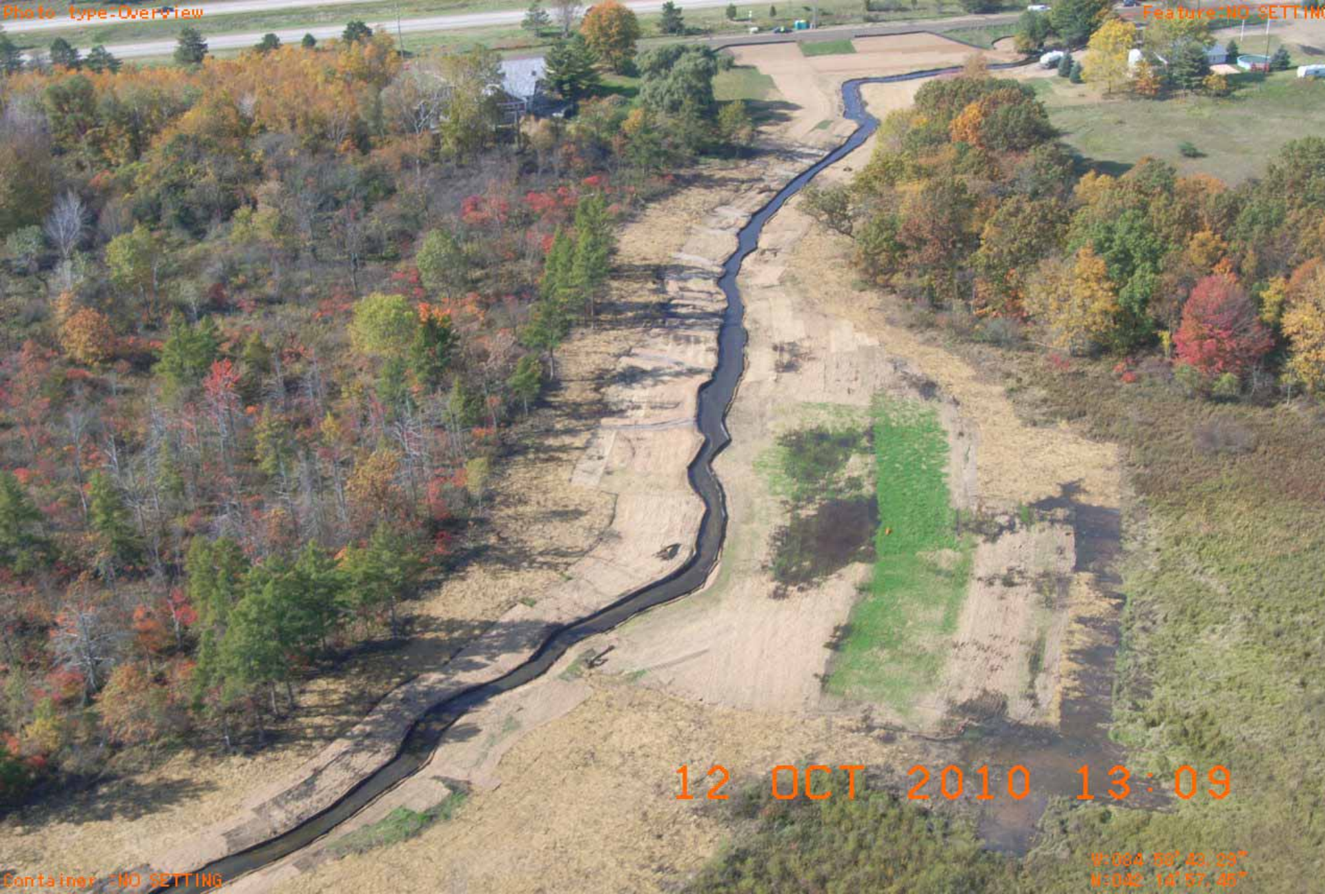
Talmadge Creek following restoration, which included soil backfilling, coconut matting, vegetation seeding, and silt fencing.
