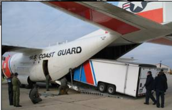
23-ft Hazmat trailer can be deployed via vehicle or C-130 aircraft
